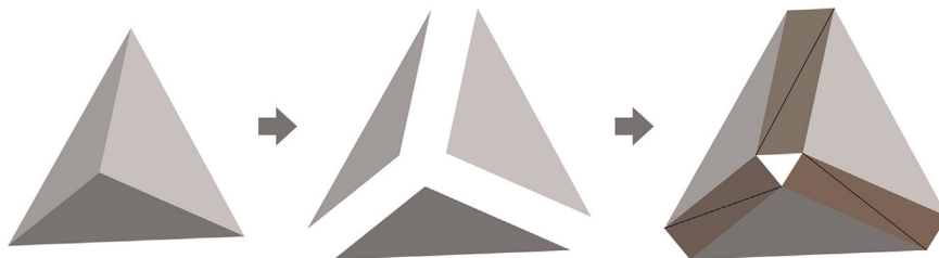
Fig. 5. Detailed illustration of mesh pre-processing, duplicating the mesh vertex, and filling in the gap by regenerating new triangles with the original four vertices.
