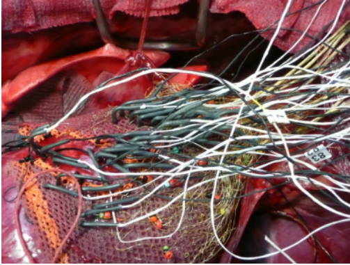
Figure 1. In situ dog heart with 247 electrode sock and 40 transmural needles inserted into the ventricular walls
