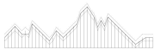
Figure 2: The solid line is calculated by a greedy method. In linking data points, go as far as possible without exiting the strip defined by the dashed lines.
