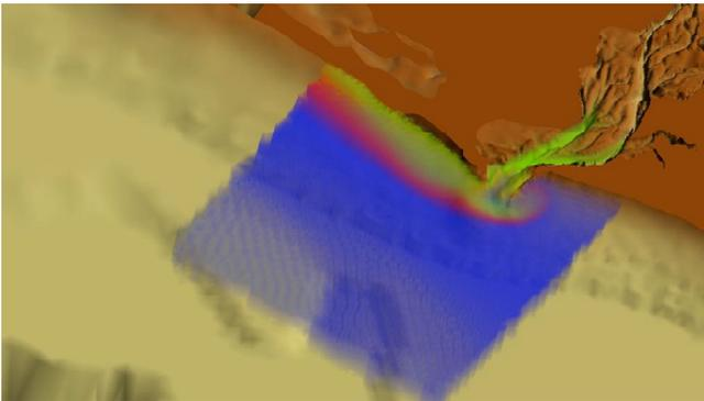
Figure 8: 3D detail of the freshwater plume during the ebb tide, showing a sharp density front (right side of the image).
