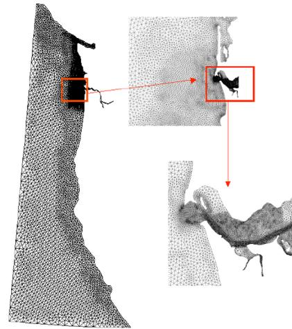
Figure 2: The CORIE computational domain extends along the continental shelf from British Columbia to California. An horizontally unstructured grid enables enhanced refinement in areas of primary interest, including the near-field plume, the estuary entrance and the navigation channel.
