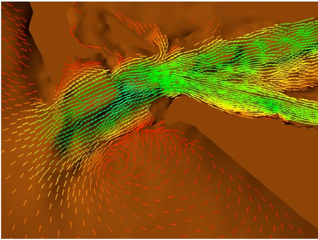
Figure 10: Instantaneous view of the velocity field during ebb tide. An eddy can be observed south of the entrance, in sharp contrast with the linear flow patterns in the channels.
