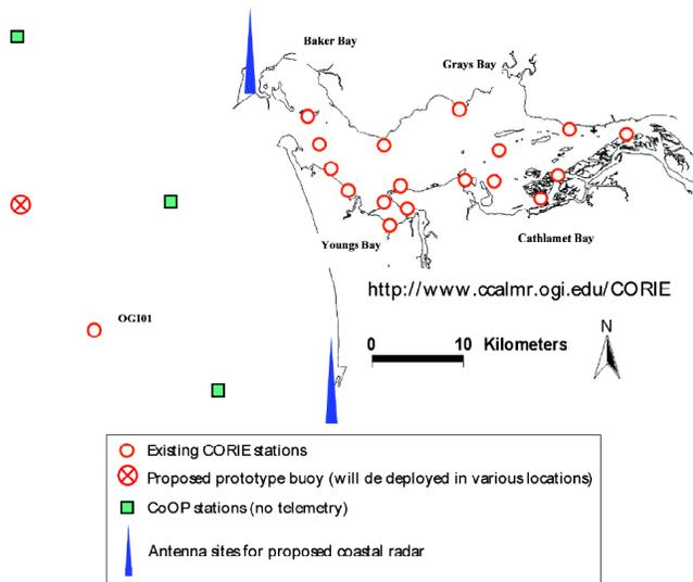
Figure 1: The CORIE observation network is an adaptive system, inherently collaborative with other programs. For instance, recently proposed CORIE stations and stations of the CoOP program are shown in the figure side by side with existing CORIE stations.
