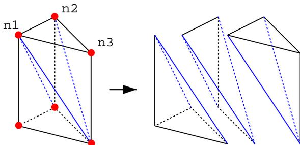
Figure 4: One wedge can be subdivided into three tetrahedra.
