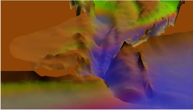
Figure 7: 3D detail of the salinity intrusion during flood tide, showing the split of ocean water entering the estuary between the Navigation Channel (at right) and the North Channel (at left). Ocean water is represented in blue, fresh water in green.
