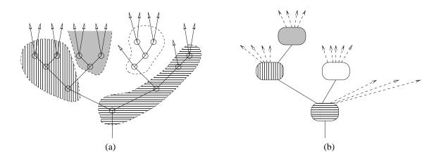
**Figure 1.** (a) A BSP tree, showing a grouping of compositing operations and (b) the corresponding tree of compositing processes. Each compositing process can be mapped to a different physical node in the parallel machine.
