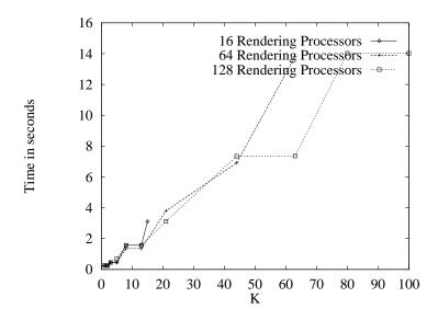
Figure 5. Variation of overall compositing time with K across the three benchmarked configurations. Notice that the compositing capacity needed increases with the number of rendering nodes. In order to keep the desired frame rate, one needs to increase the number of processors allocated to the compositing tree. By keeping K constant, this is achieved automatically, since the number of compositing processors needed also grow, and can be computed by our optimal partitioning algorithm.
