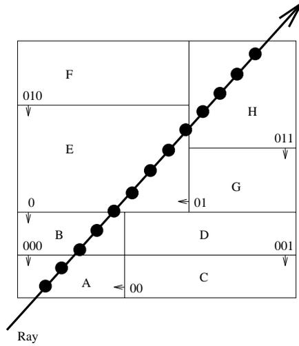
Figure 15: *Data partitioning shown in two dimensions. The dataset is partitioned into 8 pieces (marked A . . . H) in a canonical hierarchical manner by the 7 lines (planes in 3D) represented by binary numbers. Once such a decomposition is performed, it is relatively easy to see how the samples get composited back into a single value.*
