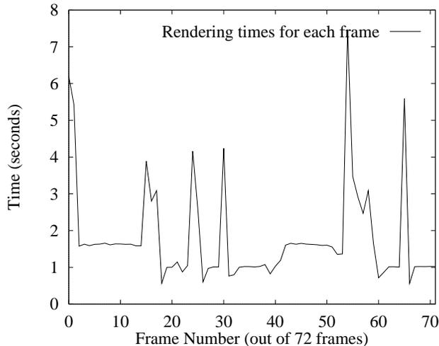
Figure 6: *Rendering times for a 72-frame animation sequence of the  $512 \times 512 \times 1877$  visible human dataset. Each image is  $400 \times 400$ .*
