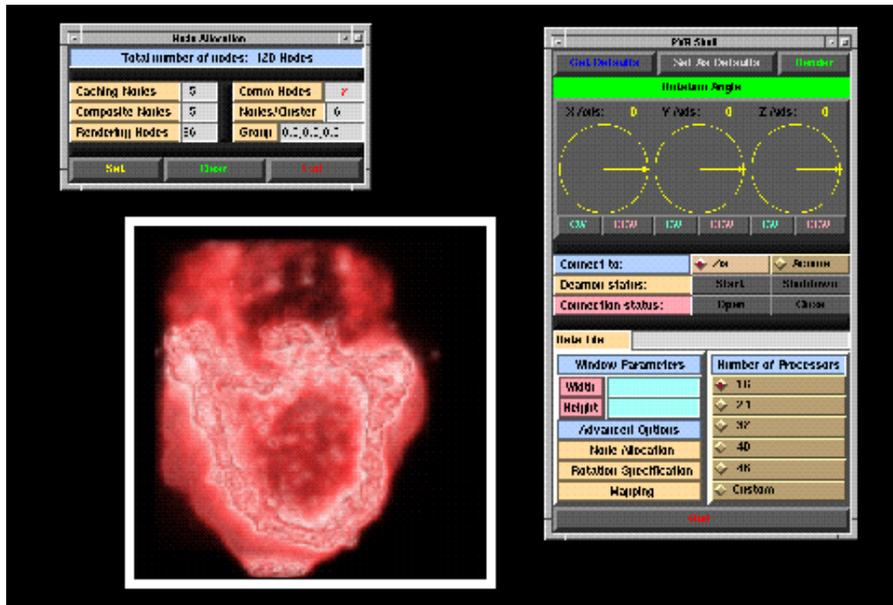
Figure 13: A snapshot of the simple PVR GUI, with three windows. The main interface window on the right, where the user can specify general rotations. The cluster configuration window, on the left. The third window is the image of a cell calculated with PVR.
