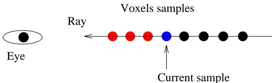
Figure 8: A typical ray is shown, together with its samples.
