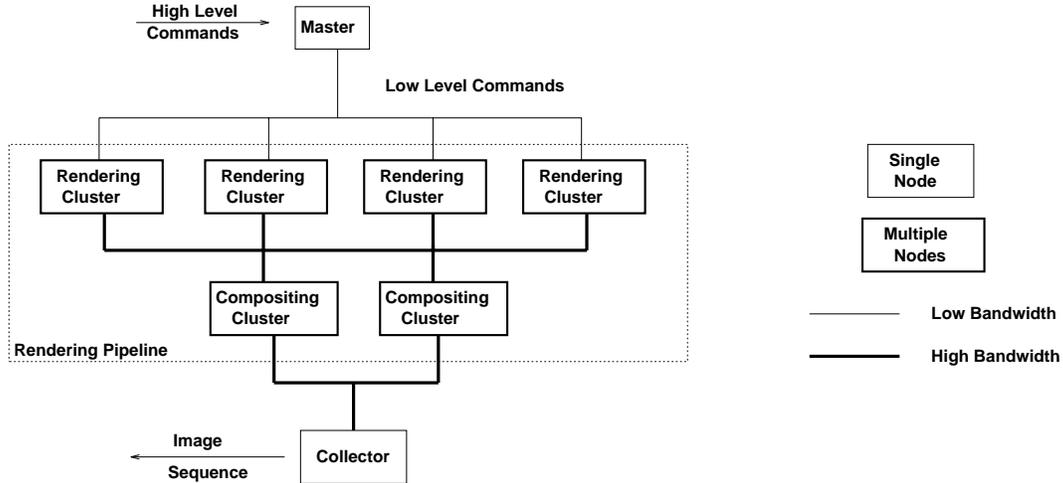
Figure 4: *The master receives high level commands that are translated into virtual microcode by the action tables. For rendering, the high level commands are for the generation of animations by rotations and translations, which are interpreted into simple transformation matrices commands. The rendering clusters perform rendering in parallel. The collector receives and groups images together and sends an ordered image sequence to the client application.*
