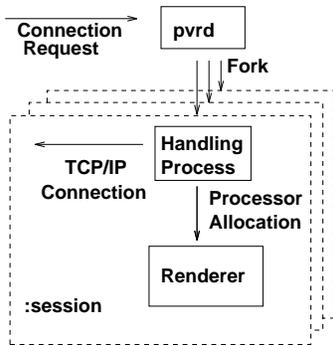
Figure 3: *In order to allocate nodes, the pvrsh sends a command to the pvr, which in turn creates a special communication handling process and allocates a partition on the parallel machine.*
