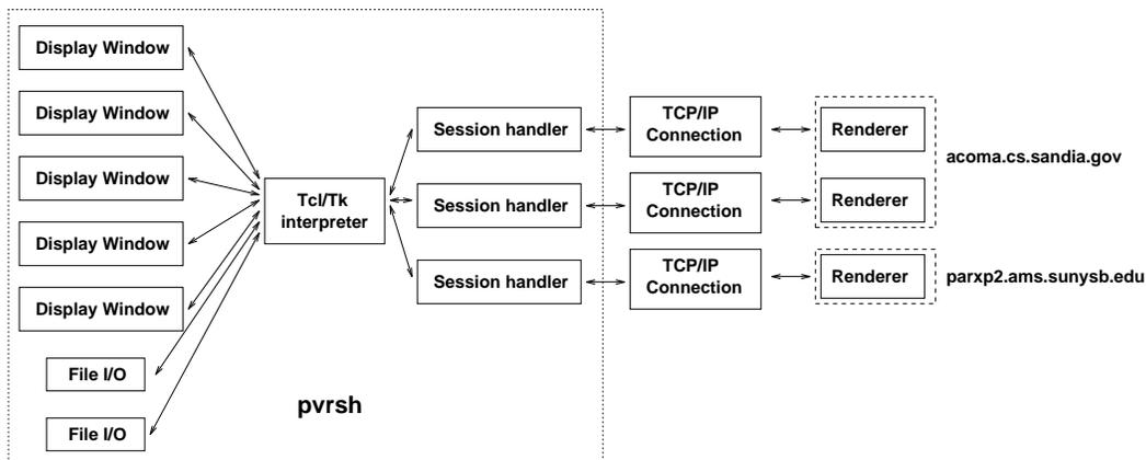
Figure 2: *PVR Architecture*. The overall structure of the system is shown with an emphasis on the *pvrsh*. The *Tcl/Tk* core acts as glue for all the client components. Everything, with the exception of the renderers, runs on the user's workstation. The renderers run remotely on the parallel machines.
