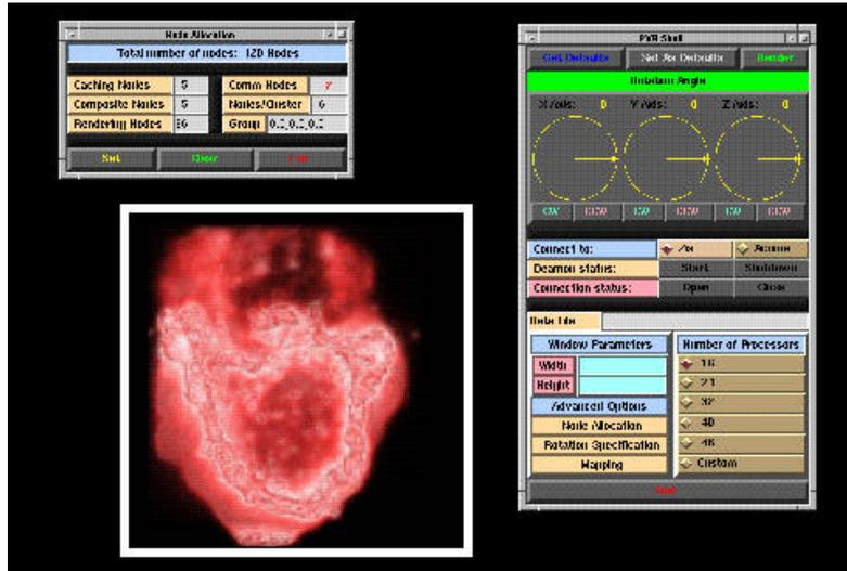
Figure 47: A snapshot of the simple PVR GUI, with three windows. The main interface window on the right, where the user can specify general rotations. The cluster configuration window, on the left. The third window is the image of a cell calculated with PVR.
