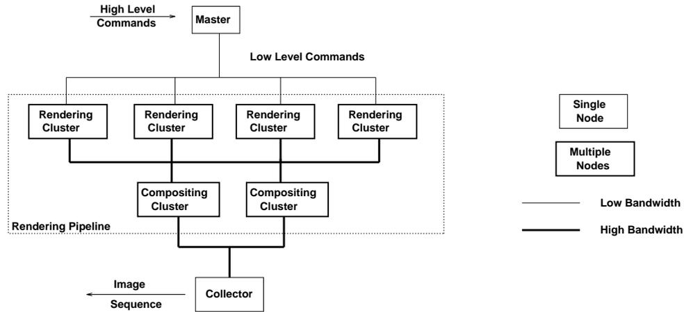
Figure 41: *The master receives high level commands that are translated into virtual microcode by the action tables. For rendering, the high level commands are for the generation of animations by rotations and translations, which are interpreted into simple transformation matrices commands. The rendering clusters perform rendering in parallel. The collector receives and groups images together and sends an ordered image sequence to the client application.*
