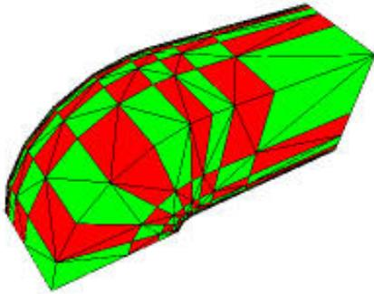
Figure 21: *Outside faces of a lower resolution version of the Blunt Fin are shown to demonstrate the tetrahedralization process. Red and green cells have to be tetrahedralized in opposite direction to allow for correct matching between cells.*
