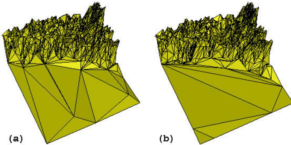
Figure 27: *Buffalo terrain triangulated with (a) Franklin's algorithm, (b) our algorithm (strong-feasibility).*
