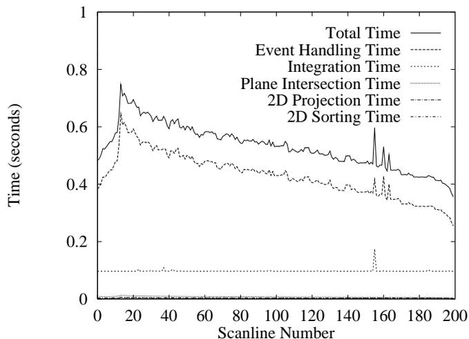
Figure 20: *Total rendering time as a function of the scanline: the intersection time is the time it takes to calculate the 2D point of intersection of the active edges with the scanplane; the event handling time is the time to process every active edge after sorting, including the 1D ray sorting necessary for integration. Note that event handling time dominates the total cost of a scanline.*
