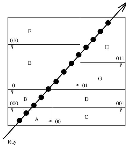
Figure 10: *Data partitioning shown in two dimensions. The dataset is partitioned into 8 pieces (marked A . . . H) in a canonical hierarchical manner by the 7 lines (planes in 3D) represented by binary numbers. Once such a decomposition is performed, it is relatively easy to see how the samples get composited back into a single value.*
