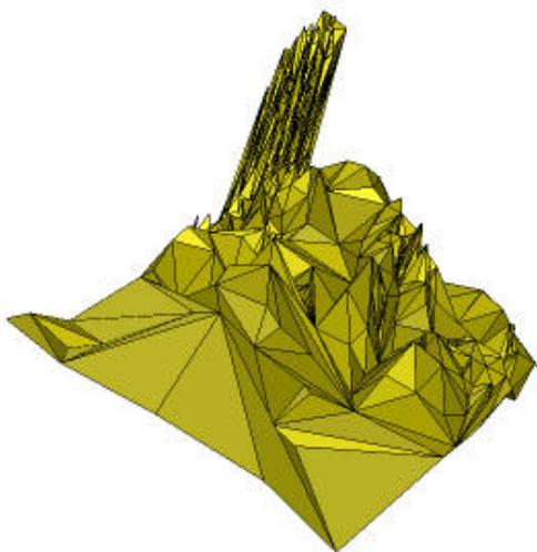
Figure 32: *Denver terrain triangulation,  $\epsilon = 5$  units.*
