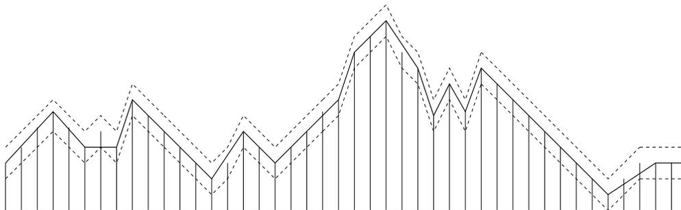
Figure 26: *The solid line is calculated by a greedy method. In linking data points, go as far as possible without exiting the strip defined by the dashed lines.*
