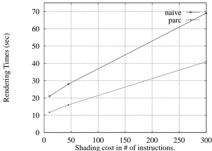
Figure 12: *PARC* versus naive ray casting. Times were calculated on a Sparc1000.
