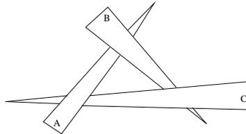
Figure 15: *3 triangles that have no depth ordering.*
