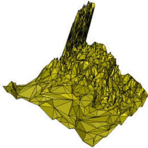
Figure 33: *Denver terrain triangulation,  $\epsilon = 2.5$  units.*
