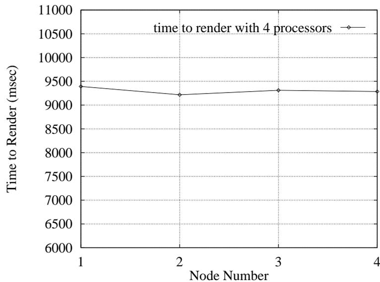
Figure 6: *Our load balancing on the Paragon. The graph shows the actual rendering times for 4 processors using our load balancing.*
