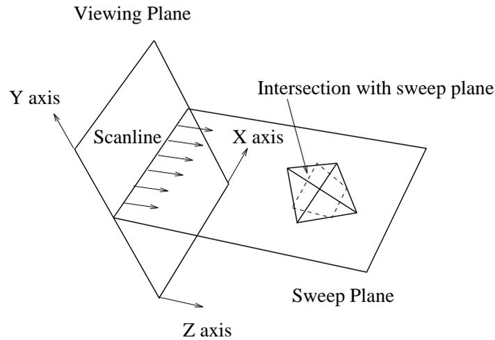
Figure 16: A sweep-plane (perpendicular to the  $y$ -axis) used in sweeping 3-space.
