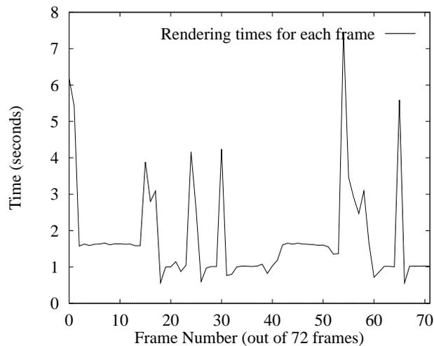
Figure 13: *Rendering times for a 72-frame animation sequence of the 512-by-512-by-1877 visible human dataset. Each image is 400-by-400.*
