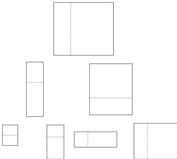
Figure 7: *An example of the partition scheme we used for load balancing. The bottom represents a possible decomposition for 8 nodes. Notice that a cut can be made several times over the same axis to optimize the shape of the decomposition.*
