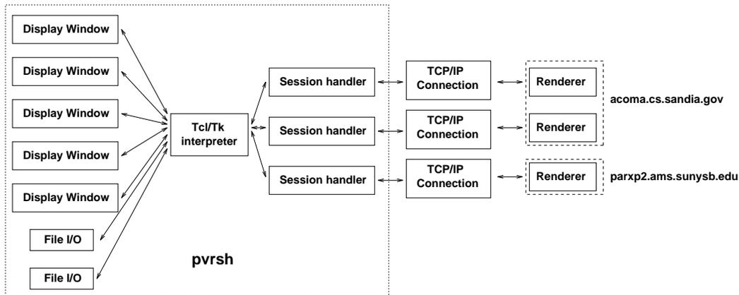
Figure 39: *PVR Architecture*. The overall structure of the system is shown with an emphasis on the *pvrsh*. The *Tcl/Tk* core acts as glue for all the client components. Everything, with the exception of the renderers, runs on the user's workstation. The renderers run remotely on the parallel machines.
