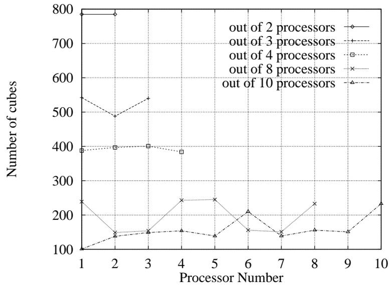
Figure 4: *Load balancing measures for our algorithm. The graph shows the number of cubes the processor receives in our algorithm.*
