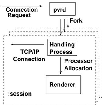
Figure 40: *In order to allocate nodes, the pvrsh sends a command to the pvr, which in turn creates a special communication handling process and allocates a partition on the parallel machine.*
