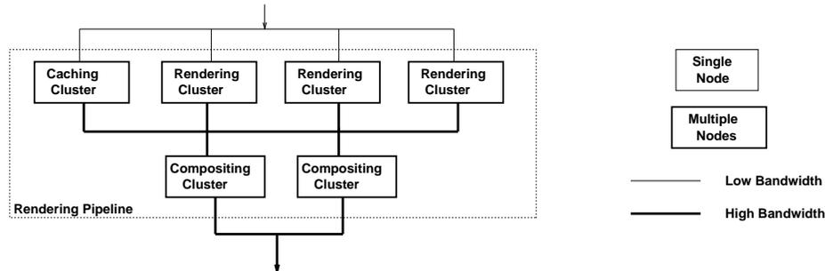
Figure 9: *Representation of the rendering pipeline. Commands come from the top into the respective clusters. Each cluster is considered as a different functional unit of the rendering process and hides its internal structure from the other clusters. Flexible configuration of the nodes into clusters, and their respective functions are provided by the PVR system.*
