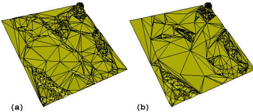
Figure 28: *Jackson terrain triangulated with (a) Franklin's algorithm, (b) our algorithm (strong-feasibility).*
