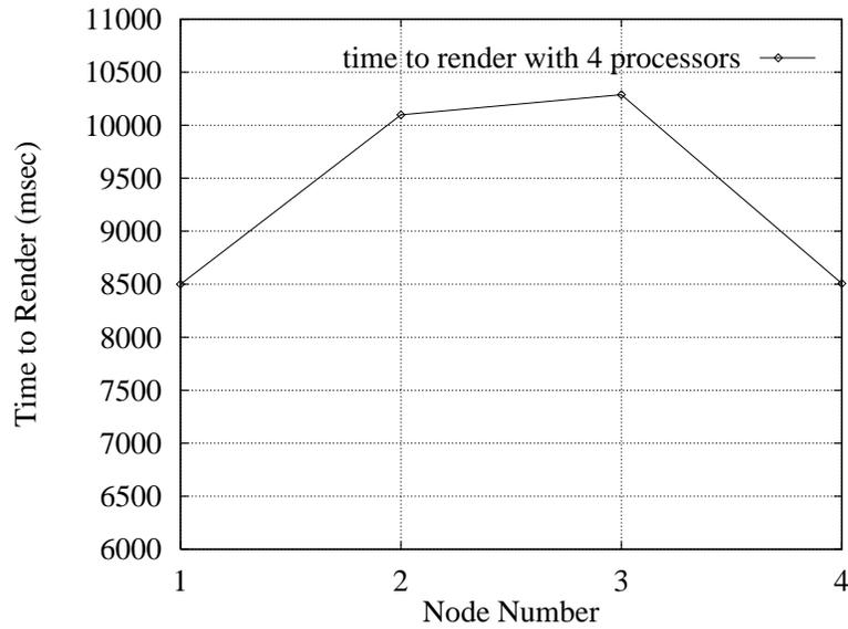
Figure 5: *Naive load balancing on the Paragon. The graph shows the actual rendering times for 4 processors using the naive load balancing.*
