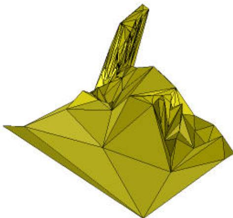
Figure 31: *Denver terrain triangulation,  $\epsilon = 10$  units.*
