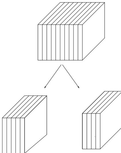
Figure 2: *During slab-based load balancing, each processor gets a range of continuous data set slabs. The number of full supervoxels determines the exact partition ratio.*
