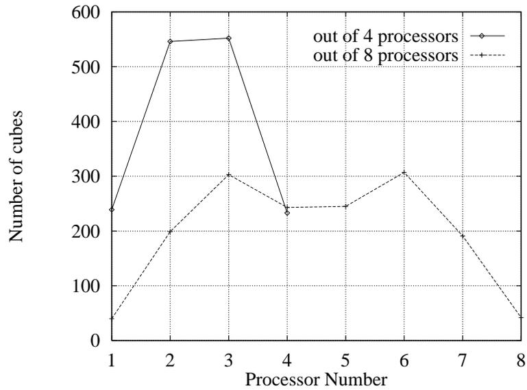
Figure 3: *The graph shows the number of cubes per processor under naive load balancing.*
