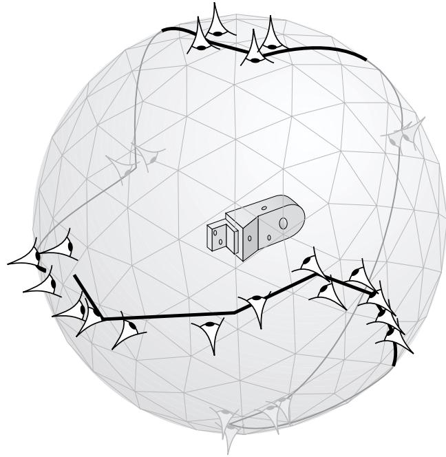
**Figure 7.12:** Planning of a stereo-sensor to inspect an object (adapted from [TUWR97])
