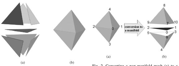
Fig. 1. The seven faces (a) composing a non-manifold mesh (b) that we will use as an example throughout this paper.
