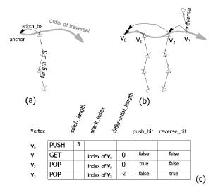
Fig. 14. Translating stitches to the bit-stream syntax.
