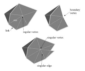
Fig. 21. Regular, boundary and singular (or non-manifold) vertices of a polygonal mesh.
