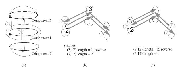
Fig. 10. Potential problems with variable-length stitches. (a) The clustering between components 1 and 2 is decoded only when component 3 is. (b) To successfully encode these two stitches we must substitute vertices 12 with 7 in the first one. (c) No possible re-combination using endpoints 3, 7 and 12 is possible.
