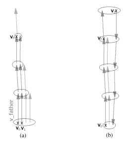
Fig. 9. Computing the longest possible stitch starting at a vertex  $v_0$ . Ovals indicate clusters. (a) Forward stitch of length 3 with  $v_1$ . (b) Backward stitch of length 4 with  $v_2$ .
