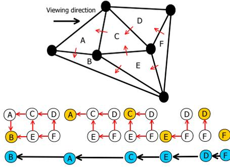
Figure 5: **MPVO algorithm**. The adjacencies define an adjacency graph. A topological sorting of this graph produces the cells in visibility ordering with respect to the viewing direction.
