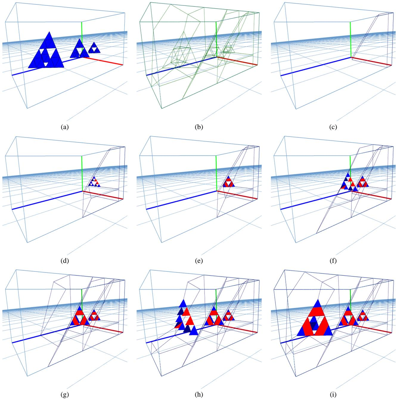
Figure 9: SF-MPVO in a dataset with disjoint parts and holes. (a) Input mesh (b) BSP-tree subdivision (c)-(i) Several instances of the algorithm showing the cells projected so far (filler meshes are drawn in wireframe)
