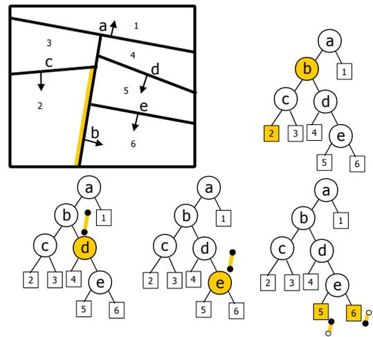
Figure 4: **Face Location algorithm example.** Find the cells adjacent to the marked face in cell 2, defined on cut  $b$ , facing the left subtree of  $b$ . Insert face in the right subtree of  $b$ . Each node tested against the face is highlighted. The test against node  $d$  passes the face to its right subtree, while against the node  $e$  splits the face in two. Leaf nodes (5, 6) reached by sub-faces are the adjacent cells.
