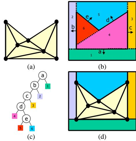
Figure 2: **BSP-Filler Algorithm.** (a) Input non-convex mesh. (b) BSP decomposition using the boundary faces of input mesh. (c) Corresponding BSP tree (d) Input mesh augmented with cells generated by the filler algorithm.
