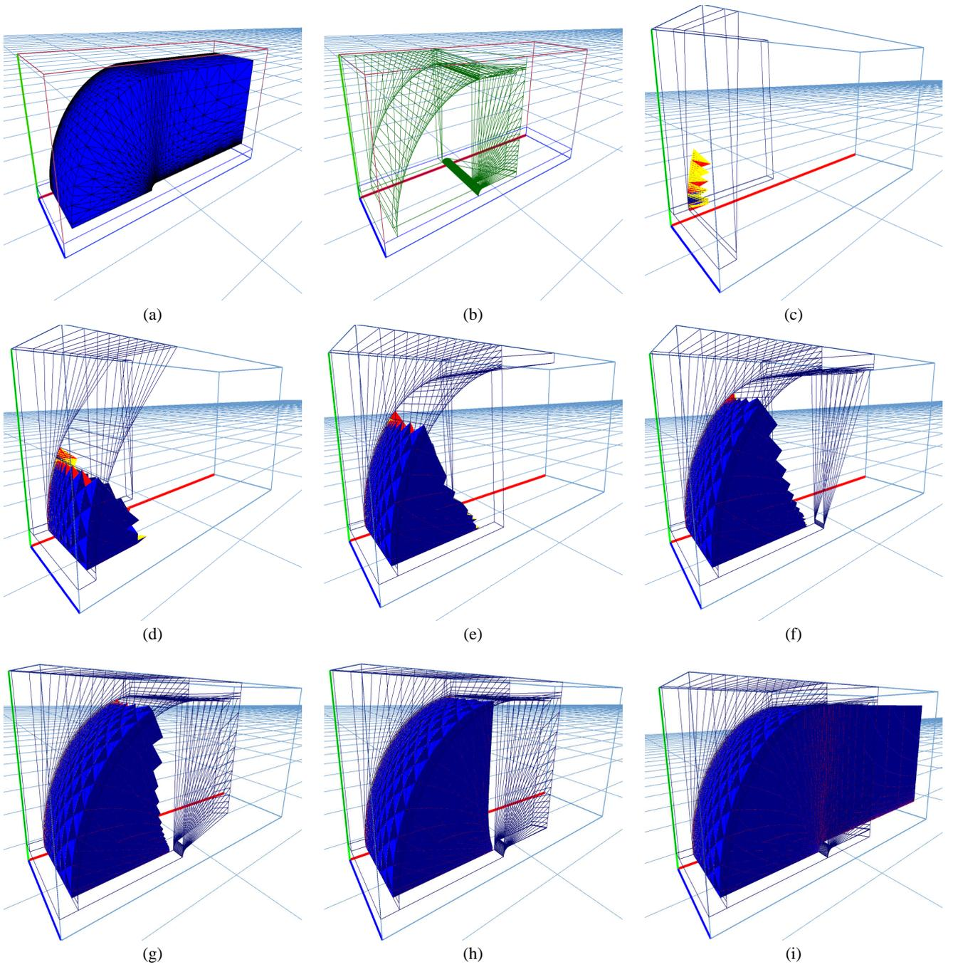
Figure 10: SF-MPVO in the BLUNT dataset. (a) Input mesh (b) BSP-tree subdivision (c)-(i) Several instances of the algorithm showing the cells projected so far (filler meshes are drawn in wireframe)
