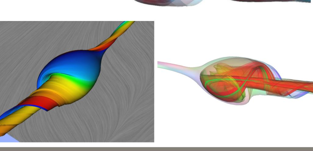
Top: Topological structure of a vortex breakdown in a simulation of a delta wing with low speed and high angle of attack. Stream surfaces in red and yellow show the separating surfaces emanating from two stagnation points that bound a so-called recirculation bubble.
