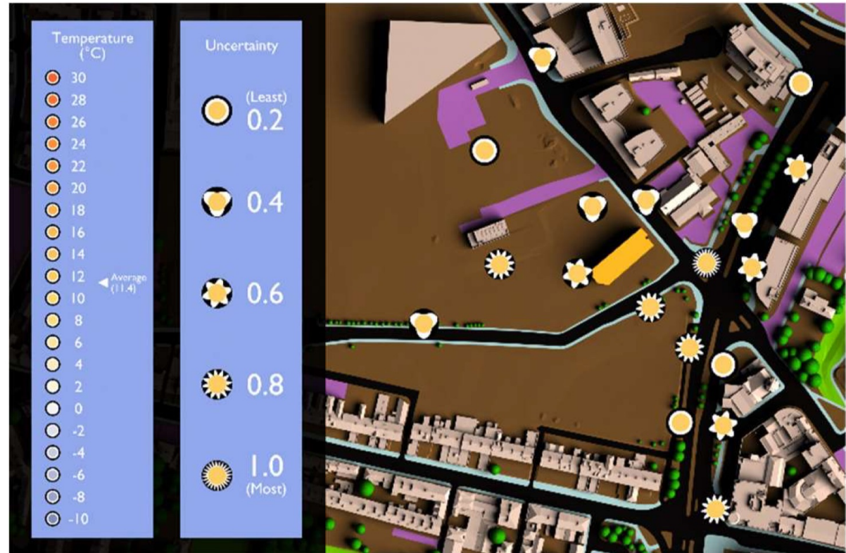
Fig. 10. The urban temperature data visualization showing both hourly mean temperature values using the MetOffice color scale and the variance of those values using our new visual entropy scale, this image is an example of the high uncertainty target-present stimulus used in the experiment described below.
