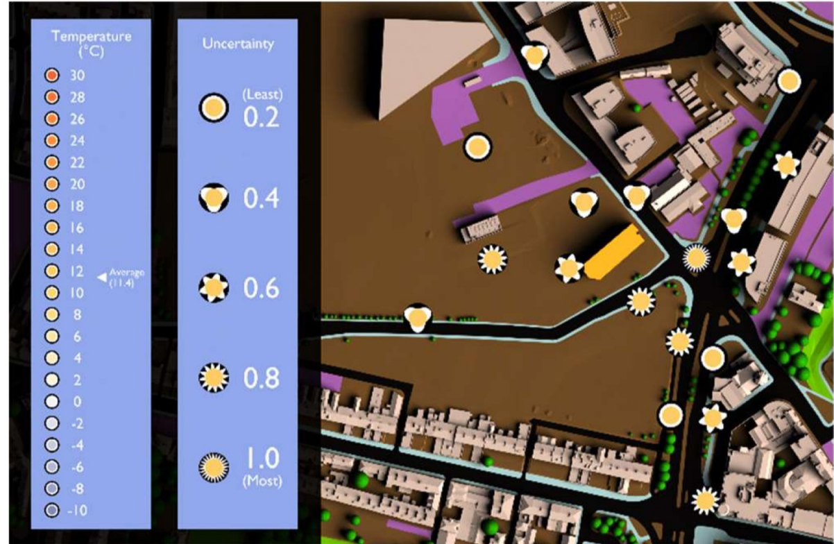
Fig. 10. The urban temperature data visualization showing both hourly mean temperature values using the MetOffice color scale and the variance of those values using our new visual entropy scale, this image is an example of the high uncertainty target-present stimulus used in the experiment described below.
