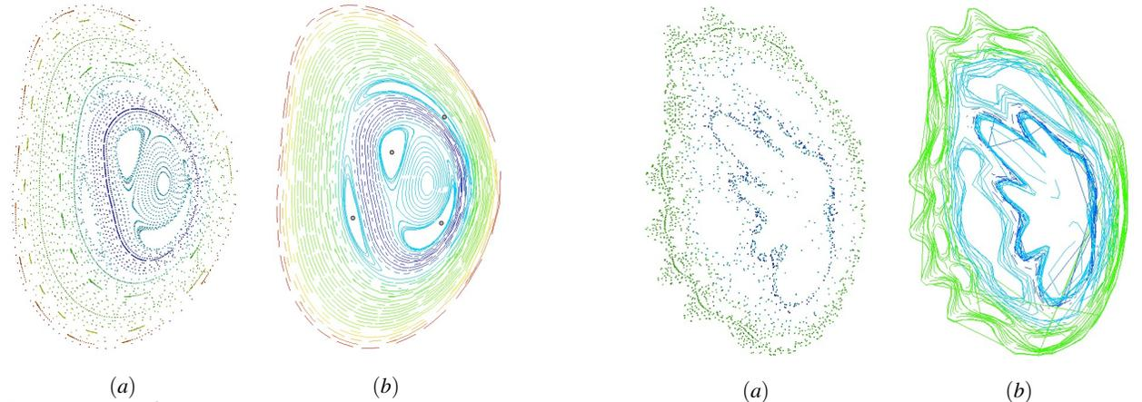
Fig. 17. The Poincaré plots of a magnetic field from NIMROD. While the inner island chain can be seen on the point based plot (a) the outer island chain is not clearly visible until the points are connected in a contiguous fashion (b).
