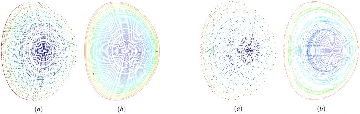
Fig. 16. The Poincaré plots of a magnetic field from M3D. There are two thin island chains, one green and one blue, that are difficult to see (a) until the points are connected and the islands identified (b).
