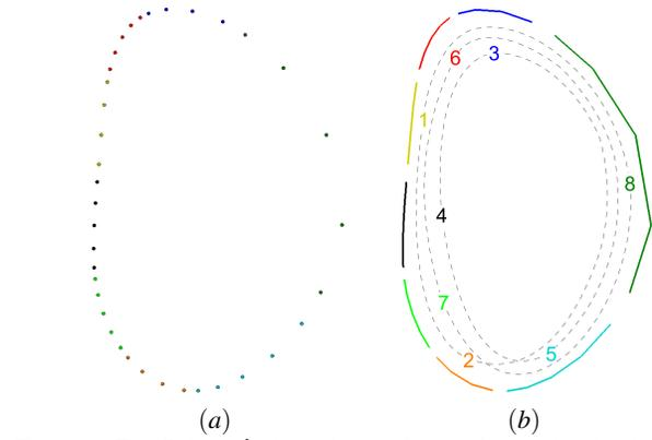
Fig. 12. The Poincaré plots of a 8,3 flux surface using (a) the original 32 points (b) the contiguous representation based on a toroidal winding number of 8. Tracing around the poloidal plane from winding group to winding group reveals the poloidal winding number of 3.
