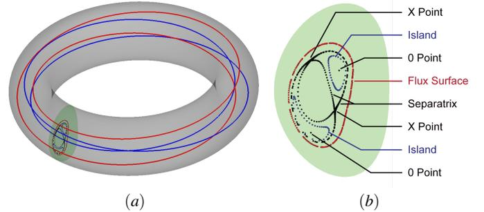
Fig. 4. (a) Two periodic fieldlines originating from an island chain's  $O$  point (red) and  $X$  Point (blue). (b) A Poincaré plot showing a flux surface (red), an island chain with two islands (blue) and their associated  $O$  points (black), and the separatrix (black).
