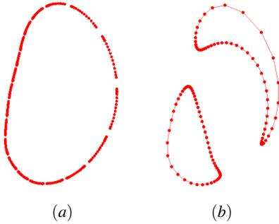
Fig. 8. (a) Poincaré section of a 19,10 flux surface. The number of curved sections, 19 corresponds to the toroidal winding number. (b) Poincaré section of a 2,1 island chain. The number of islands, 2 corresponds to the toroidal winding number. Each island contains 53 puncture points which corresponds to the fundamental period of the ridgeline plot.
