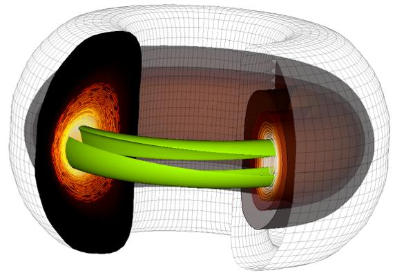
Fig. 22. A complete visualization of a magnetic confinement fusion simulation that highlights a magnetic surface (green) which forms an "island chain", along with a Poincaré plot overlaid on top of a series of transparent iso-temperature surfaces.
