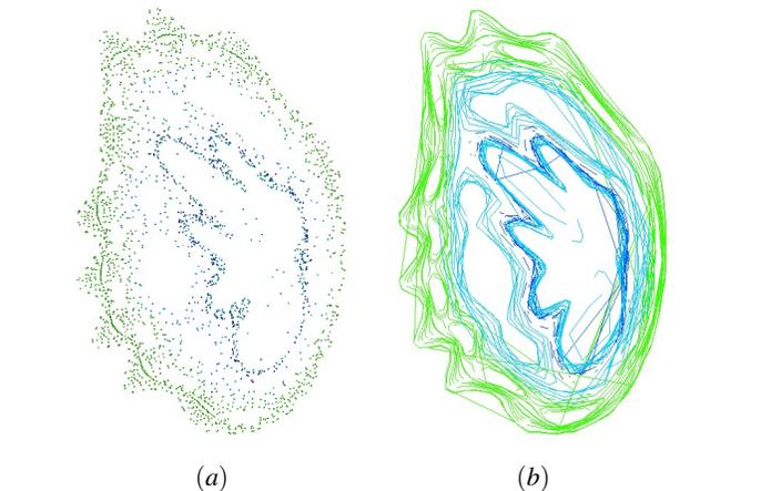
Fig. 19. A Poincaré plot of same magnetic field in Figure 17 but later in the simulation where the growth of the island chains is much more pronounced. It is difficult to discern the structure on the point based plot (a) compared to contiguous plot (b).
