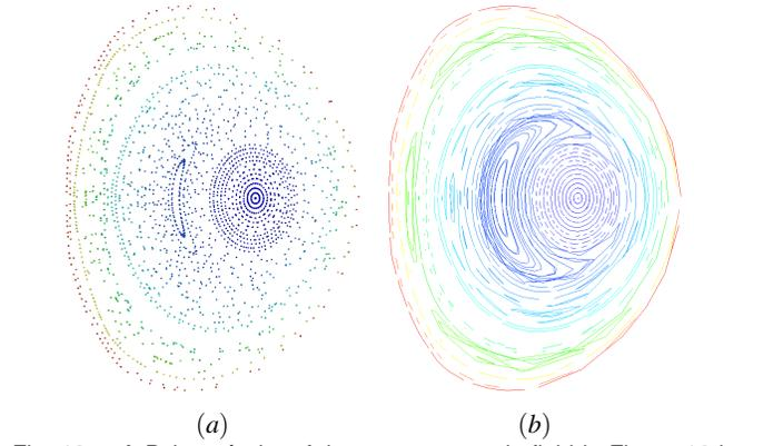
Fig. 18. A Poincaré plot of the same magnetic field in Figure 16 but later in the simulation where the growth of the island chains is much more pronounced.
