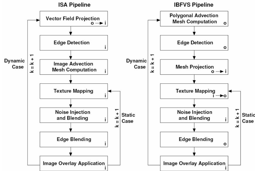
**Figure 5: The processing pipeline of the texture-based flow visualization subsystem.  $i$  indicates the operation takes place in image space and  $o$  for object space.  $o \rightarrow i$  refers to a transition takes between object space and image space, and vice versa.**
