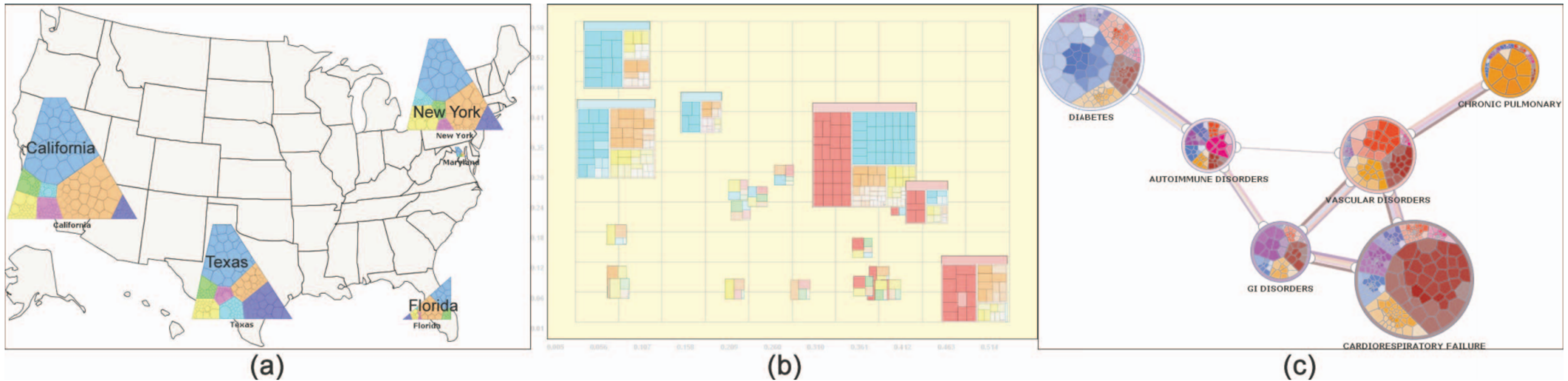
Fig. 1. DICON is a dynamic icon-based visualization technique that helps users understand, evaluate, and adjust complex multidimensional clusters. It provides visual cues describing the quality of a cluster as well as its multiple attributes, and can be embedded within many kinds of visualizations such as maps, scatter plots, and graphs.
