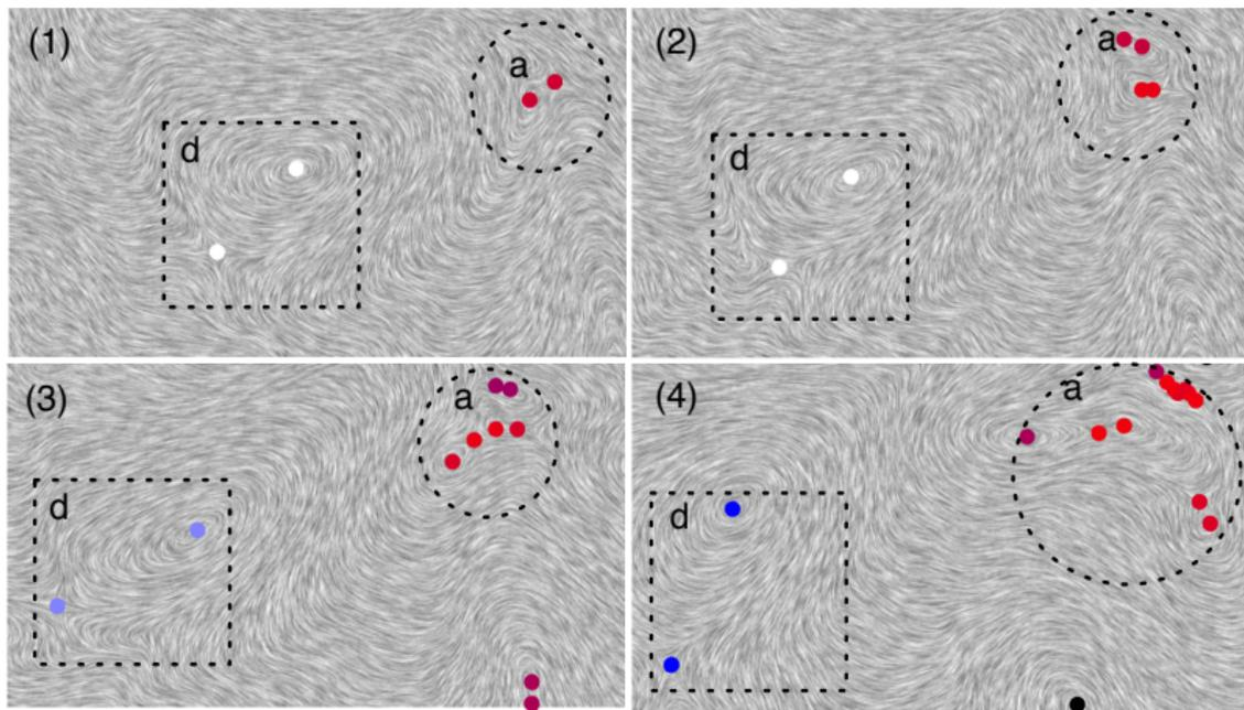
Critical points clustered by robustness for time-varying ocean eddy simulation
