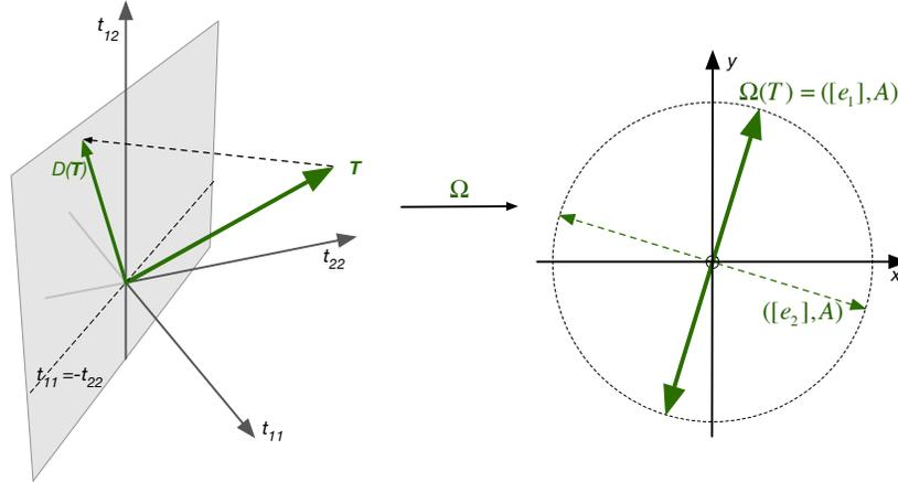
Fig. 3: Mapping of a tensor  $T$  to the bidirectional anisotropy vector defined by its anisotropy  $A$  and the eigenvector  $[e_1]$ . The space on the right represents the vector space spanned by the three independent components of the tensor. The gray plane on the left highlights the subspace of traceless tensors.
