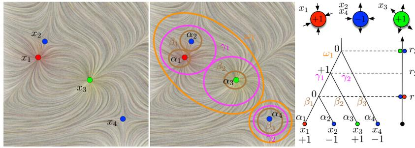
Fig. 1: Figure recreated from [28] showing the merge tree for a continuous 2D vector field example. From left to right: vector fields  $f$ , relations among components of  $\mathbb{F}_r$  (for  $r \geq 0$ ), and the augmented merge tree.  $f$  contains four critical points, a red sink  $x_1$ , a green source  $x_3$ , and two blue saddles  $x_2$  and  $x_4$ . We use  $\beta$ ,  $\gamma$ ,  $\omega$ , etc., to represent components of the sublevel sets.
