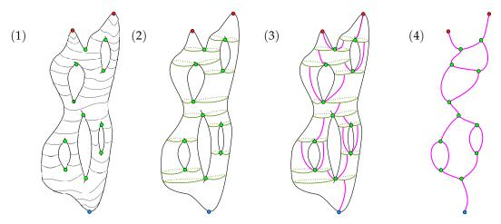
**Figure 6.** Summary of the sequential algorithm. (1) The input of the algorithm is a manifold M with a scalar function f. (2) Computing the critical sets. (3) For each saddle point or minimum, we compute the ascending paths (4) creating the edges of the Reeb graph by the information encoded in the start vertex of the ascending vertex and its termination critical set.
