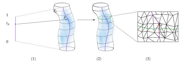
**Figure 13.** An illustration of the data retrieval procedure. (1) A value  $t_p$  is selected from the interval (0, 1). (2) This value is used to determine a point p on the Reeb graph edge  $\mathcal{E}_e$ . (3) This point is contained in an edge  $E_k$  on the mesh M. This edge is used to determine the circle  $Cr_p$
