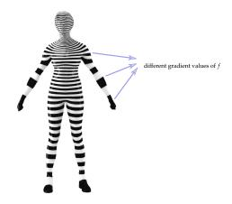
**Figure 14.** The arm of the female character mesh corresponds to a single arc in the Reeb graph associated with the scalar function indicated on the mesh. Observe that the gradient of this scalar function varies along this arm, which makes it hard to parametrize the mapping between the Reeb graph and the corresponding regions on the mesh.
