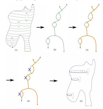
**Figure 20.** The steps of the cutting system algorithm. (1) mesh M with a scalar function defined on it are given. (2) The Reeb graph R(M, f) is computed. (3) We compute a spanning tree of R(M, f). (4) We select all edges in the graph that do not belong the spanning tree we computed in (3) and then we select an interior point on each one of these edges. (5) For each interior point, we used our augmented Reeb graph algorithm to compute the circle that corresponds to it on the mesh.
