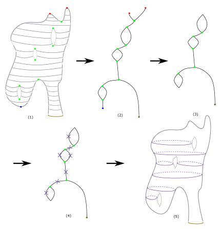
**Figure 22.** A Reeb graph can be used to segment a surface into a collection of topologically consistent patches. (1) The surface M, with a scalar function f, is given as an input. (2) The Reeb graph of R(M, f) is calculated. (3) The deformation retract graph R'(M, f) of the graph R(M, f) is calculated. (4) For each edge in the graph R'(M, f), we select a point. (5) We select the curves on the manifold M that corresponds to the points that were selected in the previous step.
