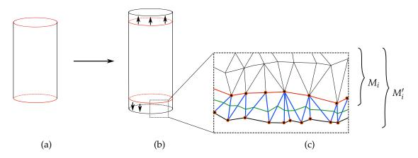
**Figure 11.** An illustration of the partition stage. (a) A connected component of the submanifold  $M_i$  is obtained. (b)  $M_i$  is extended to  $M'_i$  by adding the crossing edges. (c) A closeup of the crossing edges of the manifold  $M'_i$ . The blue edges represent the crossings edges of  $E_{i-1}$  and the green curve represents the portion of the curve  $f^{-1}(c_{i-1})$  within the closeup region.
