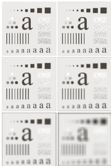
FIGURE 3.33 (a) Original image, of size 500 \times 500 pixels. (b)–(f) Results of smoothing with square averaging filter masks of sizes m = 3, 5, 9, 15, and 35 , respectively. The black squares at the top are of sizes 3, 5, 9, 15, 25, 35, 45, and 55 pixels, respectively; their borders are 25 pixels apart. The letters at the bottom range in size from 10 to 24 points, in increments of 2 points; the large letter at the top is 60 points. The vertical bars are 5 pixels wide and 100 pixels high; their separation is 20 pixels. The diameter of the circles is 25 pixels, and their borders are 15 pixels apart; their intensity levels range from 0% to 100% black in increments of 20%. The background of the image is 10% black. The noisy rectangles are of size 50 \times 120 pixels.
