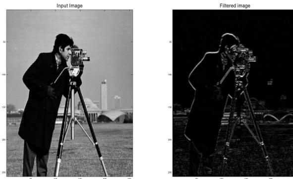
Figure 10: Cameraman image filtered with a Sobel kernel of dimension 3
