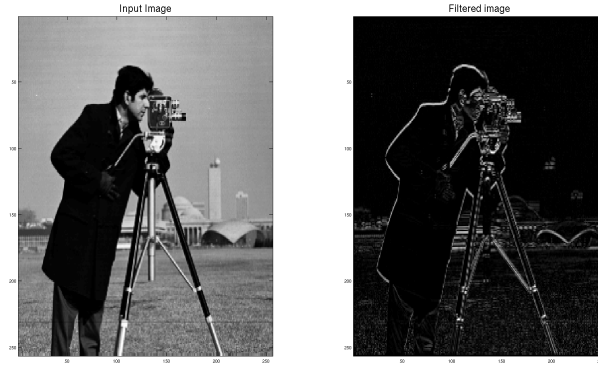
Figure 29: Detection of horizontal edges
