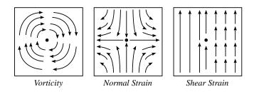
Fig. 3. Schematic views of the three components that make up the Q-criterion. Vorticity is caused by flow circling an axis, normal strain is caused by two flows colliding and pulling apart, and shear strain is caused by a lateral change in velocity.
