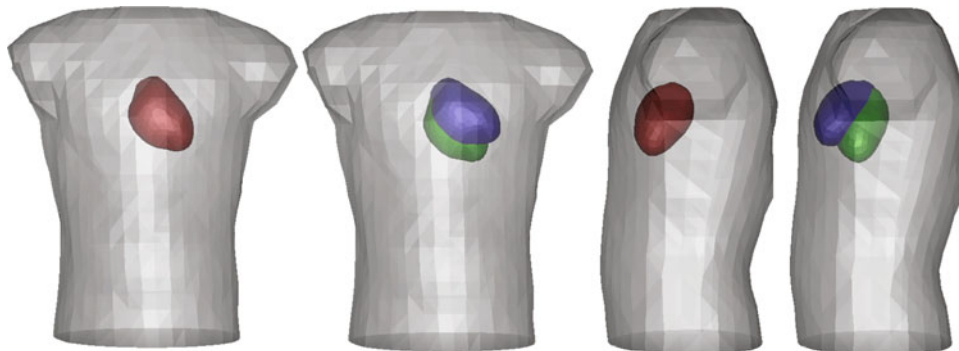
FIGURE 1. Extremes of motion of the torso tank and cardiac sources. The torso surface is grey and the epicardial surface red in the most central location. The cardiac location extremes are shown in green and blue for a pivoting motion in both x and y directions around a vector centered at the base of the heart.
