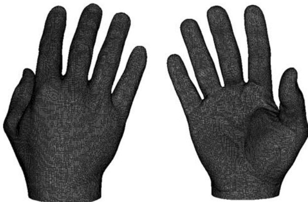
Fig. 5 Front and back view of the hexahedral mesh of the hand. The mesh contains 202,974 elements
