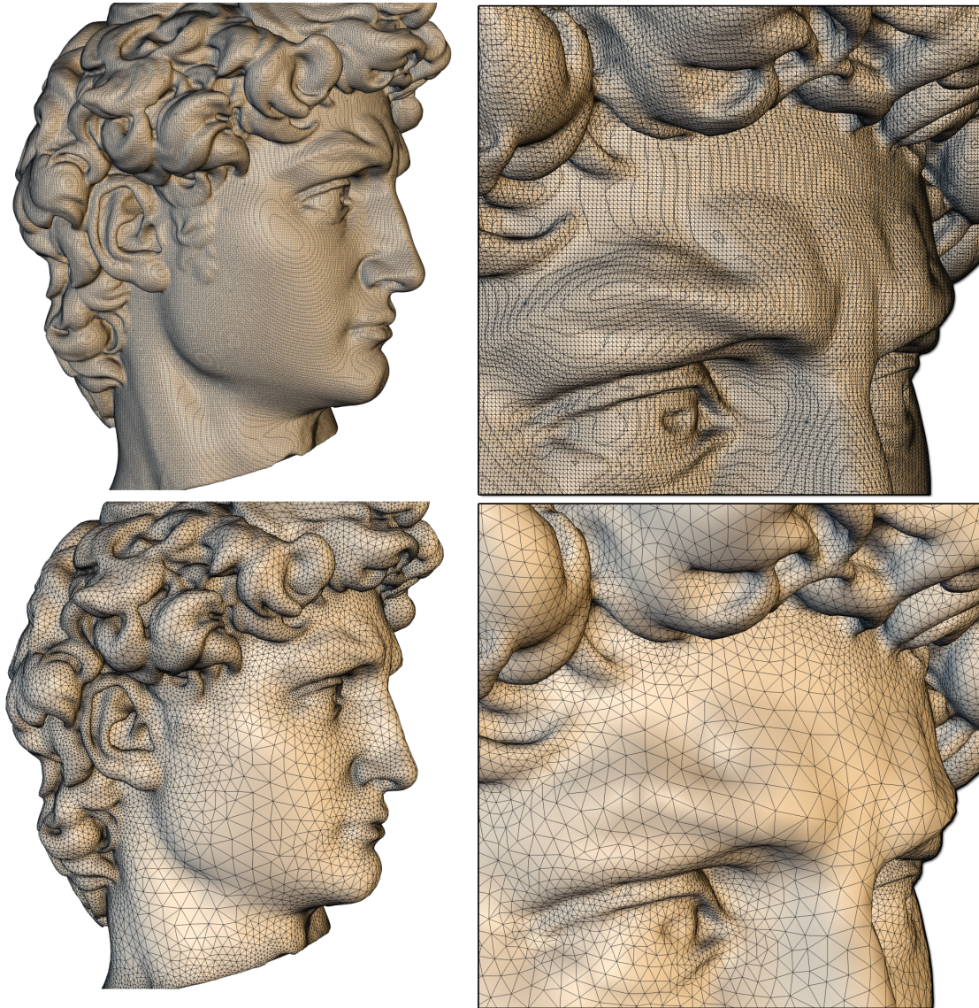
Figure 4.25: Many surface processing tasks require good meshes. At the same time, many meshes created automatically exhibit bad triangulations. The advancing front remeshing algorithm is based on surface reconstruction and requires no parameterization. The top row shows the watertight and manifold input mesh that was created with Reconstruct3D [78], and the bottom row shows a remesh generated by the advancing front algorithm.
