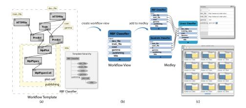
**Fig. 1.** Example of creating a medley for Example 1. (a) The developer marks configurable pieces of the workflow to create a template. (b) A workflow view is created based on the workflow template. (c) A medley of SVM Classifiers. The connections mean that synchronization is taking place.
