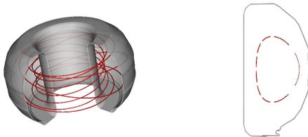
Figure 1: (a) Profile of the DIII-D Tokamak and a single quasi-periodic magnetic fieldline. (b) The corresponding Poincaré plot for the magnetic fieldline in (a) using 200 points.
