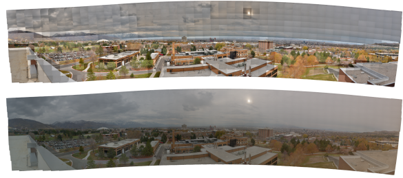
Figure 5: Fall Panorama - 126,826 × 29,633, 3.27-gigapixel. (top) The panorama before seamless blending and (bottom) the result of the parallel Poisson solver run on 480 cores with 124 \times 29 windows and computed in 5.88 minutes.
