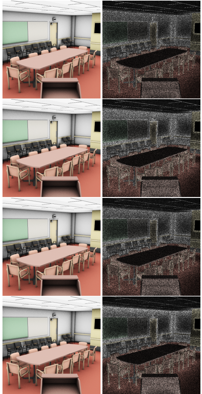
Figure 6: The Conference Room shaded with ambient occlusion, rendered using (from top to bottom) SMC importance sampling and control variates (256 spp), SMC importance sampling alone (261 spp), SMC control variates alone (258 spp), and MCMC BRDF importance sampling (274 spp) all in 43 minutes.
