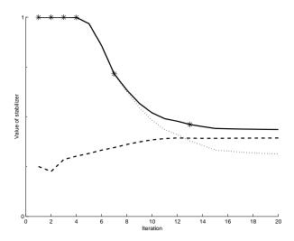
Fig. 6. Evolution of stabilizers during reweighted iterations. Solid line shows evolution of S, dashes show evolution of  $\alpha S_{reg}$  and dots show the evolution of  $(1 - \alpha)S_{min}$ . Stars show the stopping point, where term  $(1 - \alpha)S_{min}$  becomes less than term  $\alpha S_{reg}$ . After that point term  $\alpha S_{reg}$  (dashes) dominates, and  $S_{con}$  (solid line) flattens, as illustrated by this Figure.
