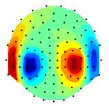
Fig. 5. Magnetic field data for two-dipole model (the model from Figure 4). Data are shown by color map superimposed on flat projection of measuring array (the helmet from Figure 3). Dots show the locations of the sensors, each sensor corresponds to one plate in Figure 3. Data contain Gaussian random noise such that the SNR=400.
