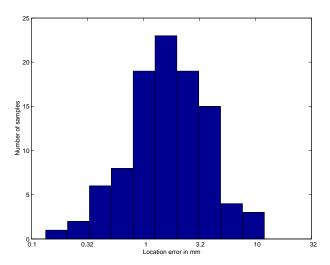
Fig. 8. Histogram of localization errors for 100 experiments with a randomly located dipole. Average error is 2.1 mm, seven errors are above 4 mm.
