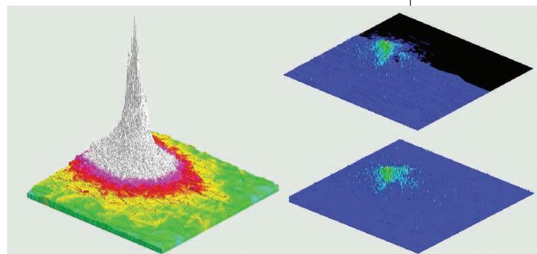
**4** Runtime memory consumption for a data set from modeling a flow field surrounding an airplane wing. The left image shows the total number of ray segments received for each pixel. The spike coincides with the fine-mesh region. The right images show the number of ray segments actually stored at two different times during the rendering. It's also apparent from the images how using a spatial partitioning tree affects the order in which ray segments are generated and delivered.
