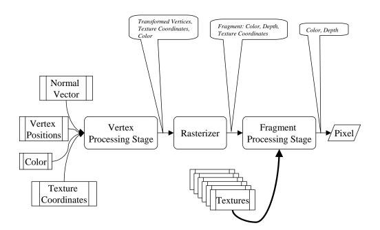
Figure 1: The graphics processing unit (GPU) pipeline.
