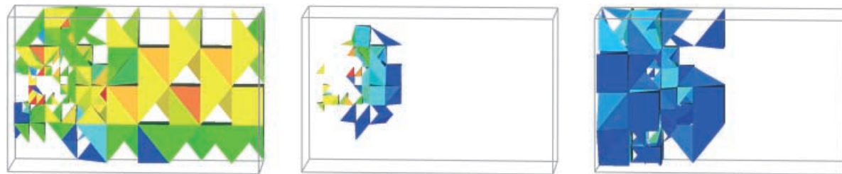
Fig. 12. Comparison of the elements flagged by three different indicators (for NO, SNGN and a tracer) used for the atmospheric model. In each figure, all elements with error values within 98% of the maximum error value are drawn. The same color map is used for all ranges and is applied to the entire scalar range in each case. The spatial distribution of error is visibly different, as is the numeric distribution of error values apparent in color patterns
