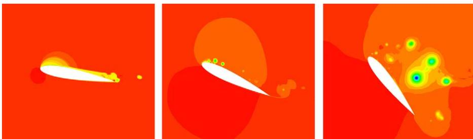
Fig. 12. Density contours for angles of attack  $\alpha = 10.4$  (left),  $\alpha = 26.1$  (center), and  $\alpha = 52.2$  (right).
