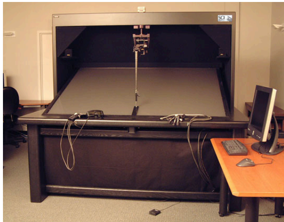
Figure 1: The Visual Haptic Workbench comprises a large workspace PHANToM mounted on top of an Immersive Workbench.
