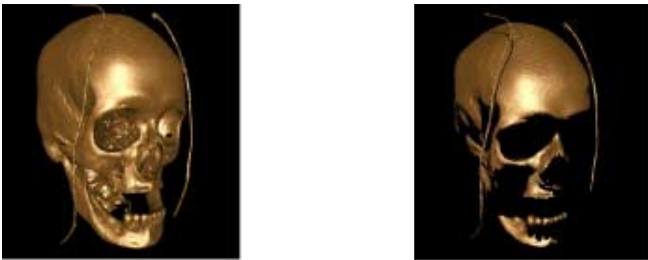
Figure 16: Full vs. View dependent isosurface extraction. The isosurfaces were computed based on a user point of view which was above and behind the skull. These images illustrate the large portions of the isosurface which the view dependent algorithm was able to avoid.
