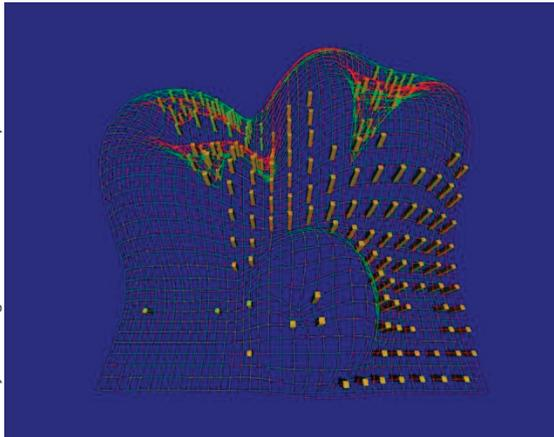
**1** Visualization of the uncertainty between two surface interpolants using displacement glyphs.
