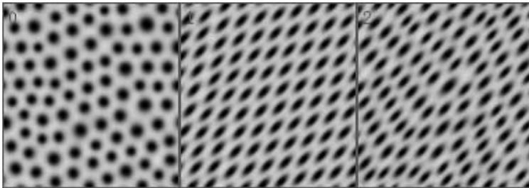
8 Gray-Scott model visualization of a vector field with (a) random magnitude, (b) constant orientation, and (c) magnitude and orientation.
