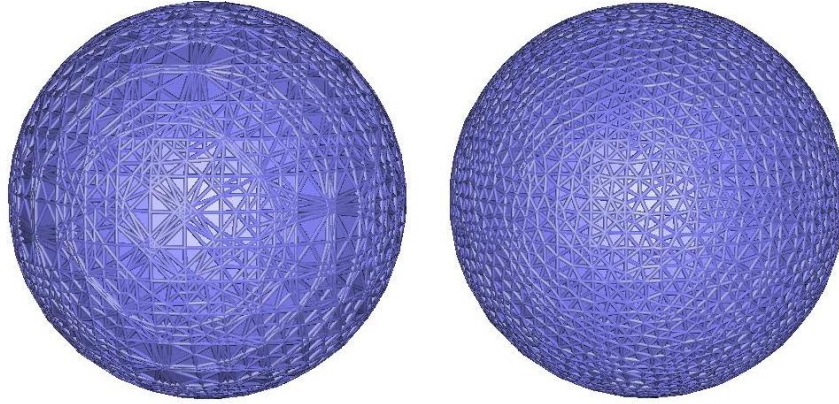
Fig. 9: Example of smart Laplacian smoothing (from the MESQUITE toolkit implemented in SCIRun) on a tetrahedral mesh. The image on the left shows the mesh before smoothing, and the images on the right is the same mesh after smoothing.
