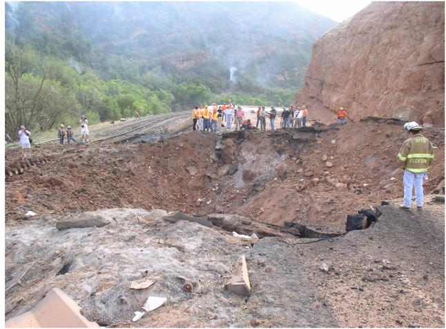
**Figure 1:** A 24 meter wide crater produced from an unexpected deflagration-to-detonation transition of 16,000 kilograms of high explosives carried by a truck through Spanish Fork Canyon, Utah.
