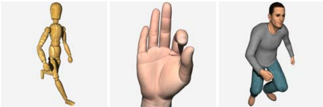
Figure 9: Some of the simpler animated models: a rigid-body wood-doll (5.3k triangles), a gesturing hand (16k triangles), and a running poser figure (78k triangles). Without shading and shadows, these scenes render at 66.9, 35.9, and 16.3 frames per second (including grid rebuild), and still at 35.1, 15.9, and 8.9 frames per second with shading, texturing, and shadows turned on.
