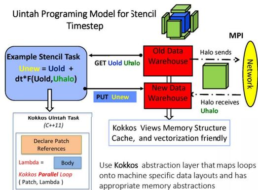
Fig. 1. Modified Uintah Programming Model
