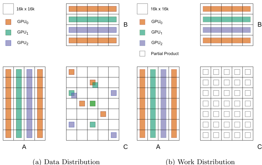
Fig. 1: Fig. (a) represents the data distribution. For each GPU, only 1 column of tiles from A and 1 row of tiles from B are considered at a time. For matrix C, each GPU gets p partial product tiles (reusable), for storing the partial GEMM computations. Fig. (b) represents the work distribution on the GPUs. It is quite similar to the data distribution, where each GPU calculate the partial result for all the elements in matrix C.
