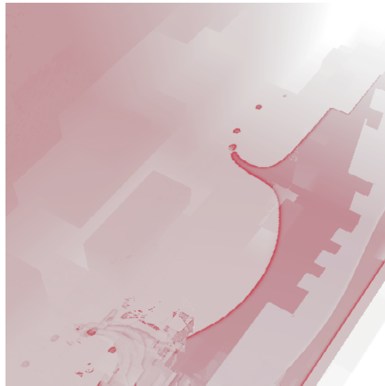
Figure 5.3. A zoomed-in view of the STP dataset (about 25M tetrahedra) captured during interaction. Significant performance improvements are made by frustum-culling the geometry on the server. Here, 50% of the geometry is culled during the progression.
