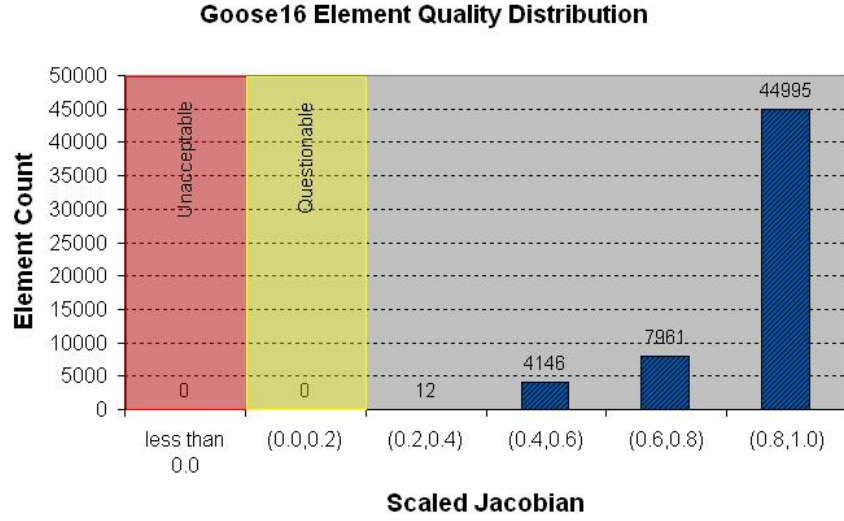
Fig. 38. Distribution of element quality for the goose16 model.
