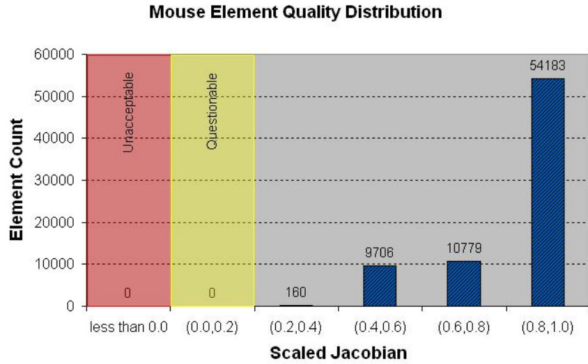
Fig. 10. Distribution of element quality for the mouse model.
