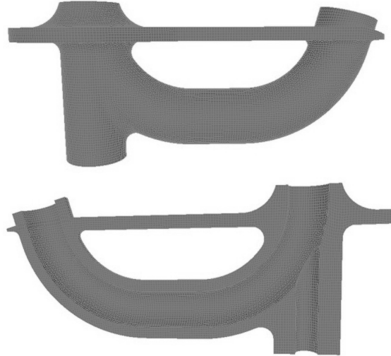
Fig. 37. Hexahedral mesh of the goose16 model showing images from the front and back of the mesh, respectively.
