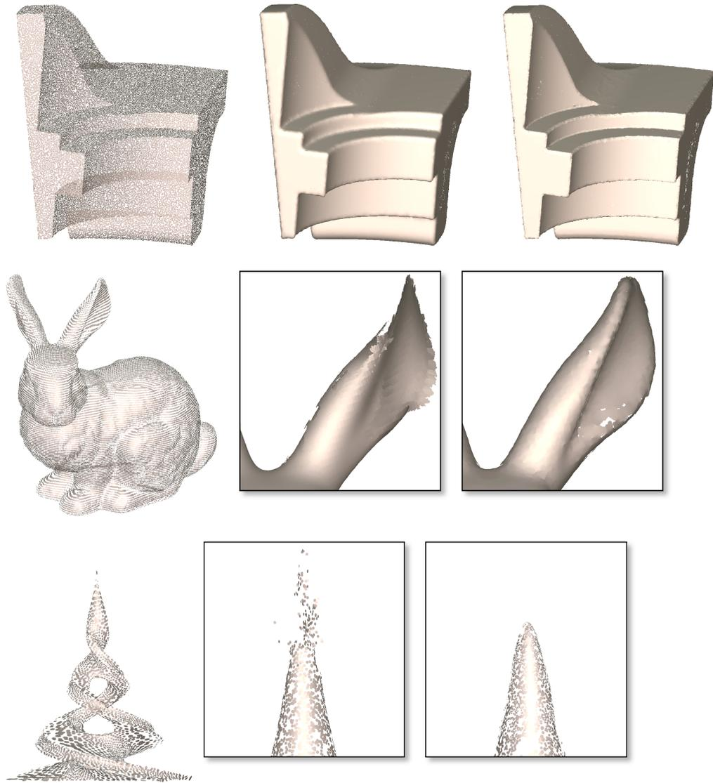
Figure 8: On reasonably well-behaved models like the fandisk (first row), our formulation (right columns) performs similarly to Levin’s (middle column). On an under-sampled point set of the Stanford bunny, or the Twirl model, Levin’s projection produces degeneracies, while our direct fitting generates an appropriate surface.
