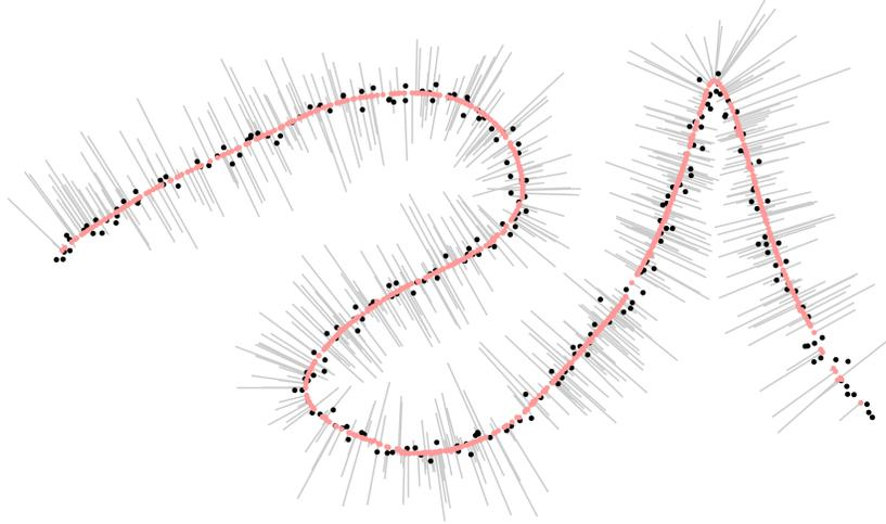
Figure 3: Like the original MLS, our unified projection is quite resilient to noisy and irregularly sampled inputs. Our approach has the extra benefit of properly rounding sharp corners. The grey lines show the paths of the point projections.
