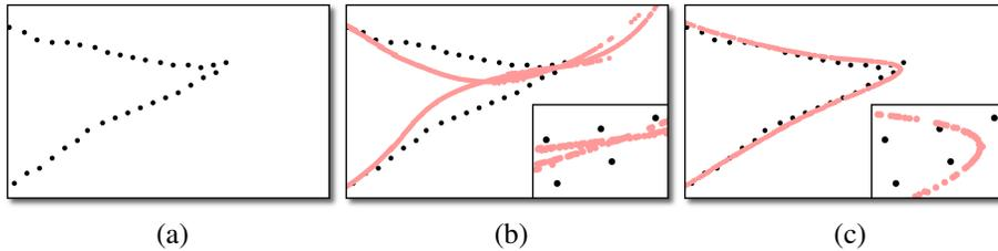
Figure 1: When Levin’s original MLS projection [Lev03] is applied to a wedge shaped set of input points (shown in black) (a), the resulting surface (shown in red) can pinch in an undesirable way as seen in (b). The surface pinches because the local reference frame bisects the input points (see Figure 4), which does not allow a good functional approximation to the points. Our new unified projection operator avoids this pinching artifact and rounds the surface as one might expect (c).
