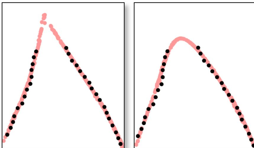
Figure 7: A function space  $\mathcal{F}$  that contains predetermined priors that fit the original surface can be used to complete missing details. On the left,  $\mathcal{F}$  contains wedge shaped functions, so a sharp point is reconstructed to fill the gap. On the right,  $\mathcal{F}$  only contains smooth functions, so the gap is filled with a smooth reconstruction.
