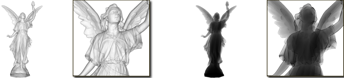
Figure 1: Example effects using the k -buffer for multi-fragment processing. The Lucy model (28,055,742 triangles) is rendered with transparency on the left and with translucency on the right. These effects captured 8 fragments per pixel in a single geometry pass and were rendered with a current hardware implementation that avoids read-modify-write hazards. With our proposed extension to hardware, these hazards can be automatically avoided and performance improved.
