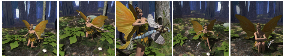
Fig. 1. Screenshots from an animated 180,000 triangle scene with moving dragonfly, fairy, and plants. At 1024 \times 1024 pixels the animated scene is ray traced at roughly 3.7 frames per second on a dual-2.6 GHz Opteron desktop PC including shadows and texturing.
