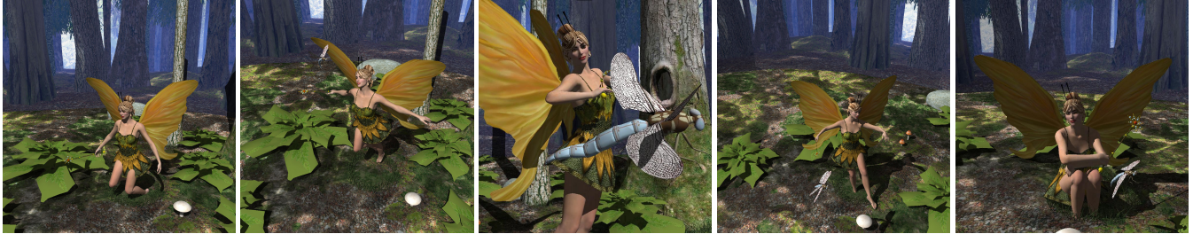
Figure 1: Screenshots from an animated 180,000 triangle scene with moving dragonfly, fairy, and plants. At 1024 \times 1024 pixels the animated scene is ray traced at roughly 3.7 frames per second on a dual-2.6 GHz Opteron desktop PC including shadows and texturing.
