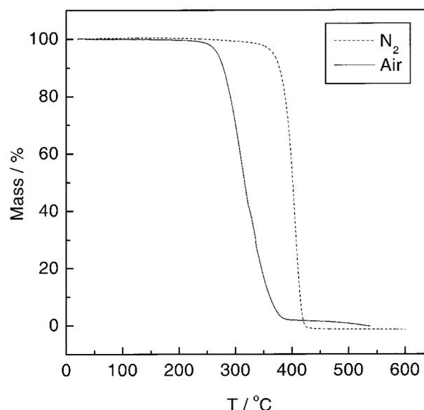
Figure 1. TGA curves for the thermal decomposition of PS in nitrogen (dashed line) and air (solid line). Heating rates of  $9.0$  and  $8.2 \text{ K} \cdot \text{min}^{-1}$  for nitrogen and air, respectively.
