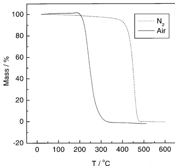
Figure 3. TGA curves for the thermal decomposition of PP in nitrogen (dashed line) and air (solid line). Heating rates of 9.1 and 8.2  $\text{K} \cdot \text{min}^{-1}$  for nitrogen and air, respectively.
