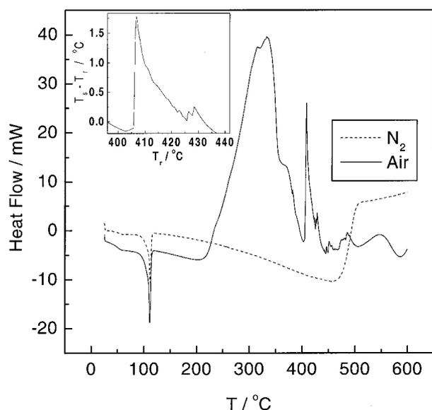
Figure 5. DSC scans of measured heat flow for degradation of PE in nitrogen (dashed line) and air (solid line). Heating rates of  $20.0 \text{ K} \cdot \text{min}^{-1}$  for both nitrogen and air. Inset plot show the difference between sample temperature,  $T_s$  and reference temperature,  $T_r$ .
