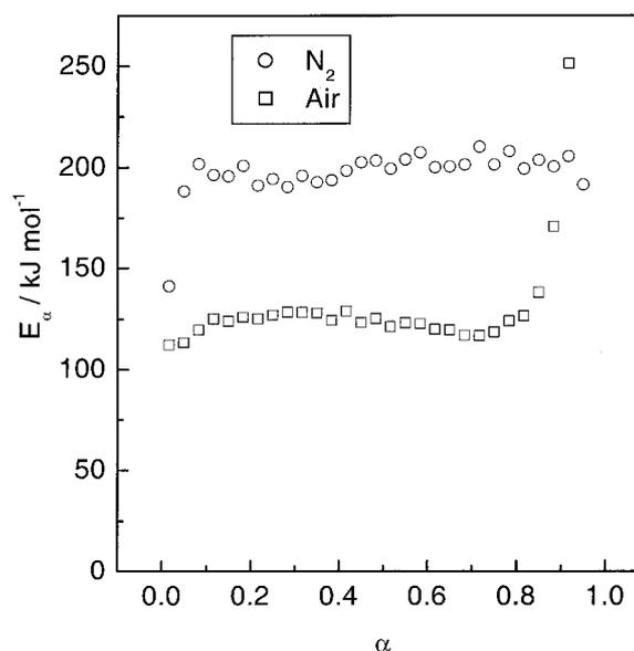
Figure 7.  $E_a$ -dependencies obtained by isoconversional analysis of TGA data for PS degradation in nitrogen (circles) and air (squares).
