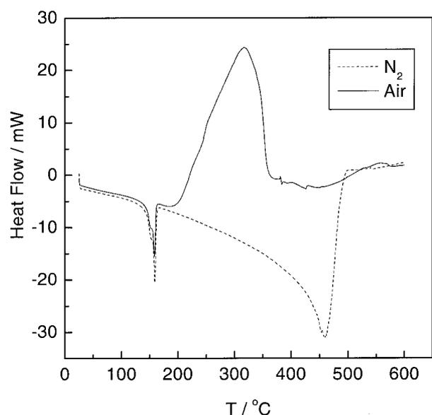
Figure 6. DSC scans of measured heat flow for degradation of PP in nitrogen (dashed line) and air (solid line). Heating rates of  $20.0 \text{ K} \cdot \text{min}^{-1}$  for both nitrogen and air.
