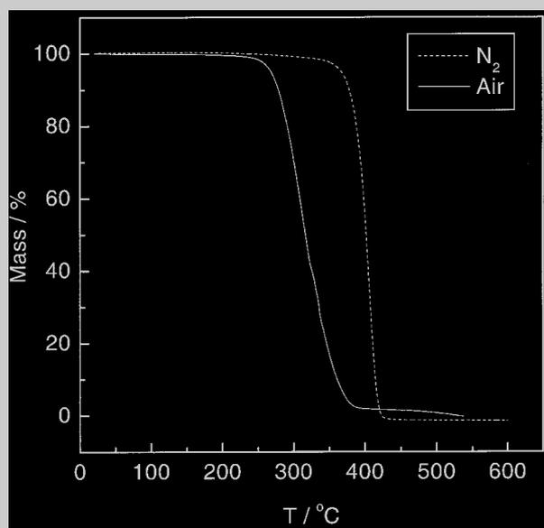
TGA curves for the thermal decomposition of PS in nitrogen (dashed line) and air (solid line). Heating rates of 9.0 and 8.2  $\text{K} \cdot \text{min}^{-1}$  for nitrogen and air, respectively.
