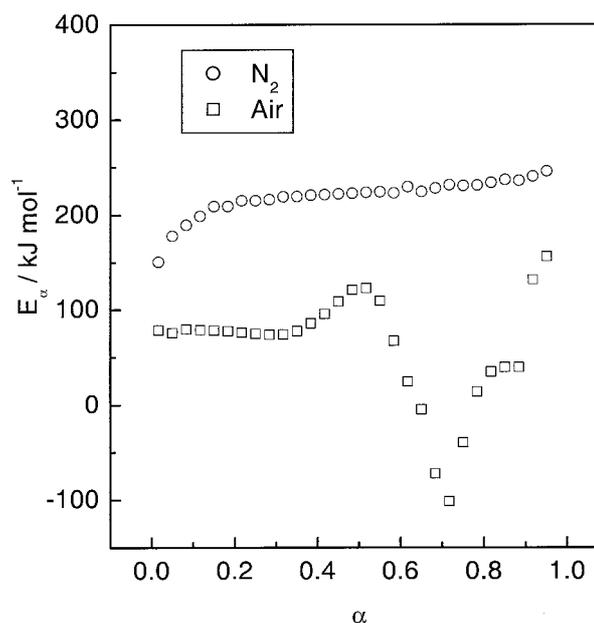
Figure 8.  $E_a$ -dependencies obtained by isoconversional analysis of TGA data for PE degradation in nitrogen (circles) and air (squares).
